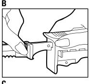
**IMPORTANT:** Unplug and be sure the Safety Button is in the "Lock" position before inserting or removing Blades. In this position, the Operating Bar cannot be pressed in even when the Knife is plugged in. (A).
